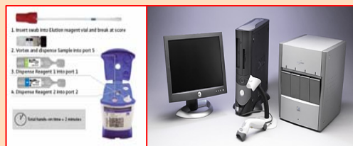
Figure 1: Xpert MRSA cartridge, reagents and the 4-site GeneXpert system
